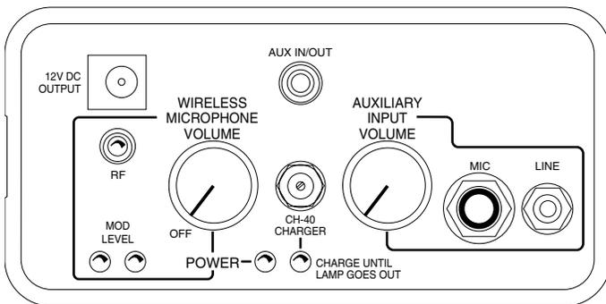
Figure 1 - Long Ranger III Control Panel
